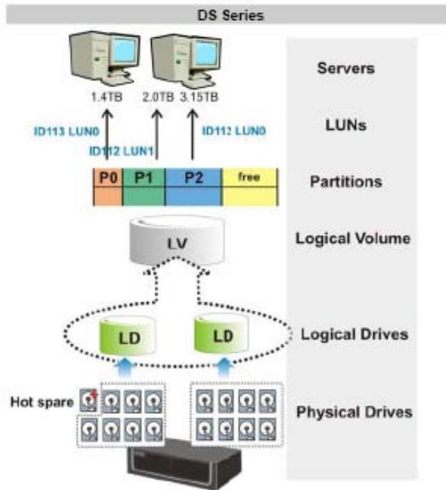
On the HA3969 high-density solutions, the drawer design adds some extra variables to LD deployment. In particular, L should not exceed the size of one drawer, i.e. 16 disk drives.
