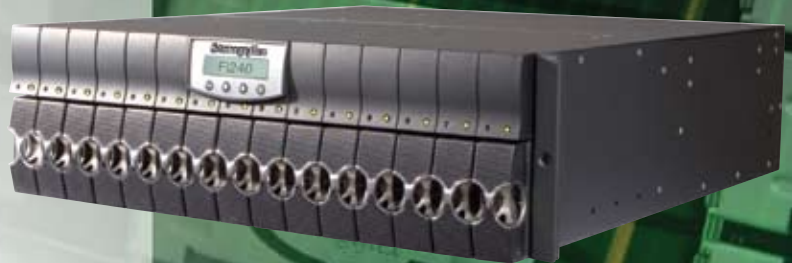
Photo of Main RAID Controller (Dual Controller Optional) with 15 Hot Swap Disk Bays expandable to 240 Disks
